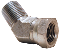
45° male NPTF x female NPSM swivel
