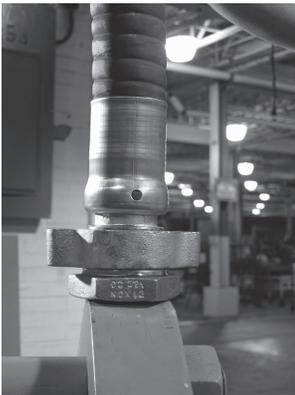
Wipe excess lubricant from hose and ferrule. Bring hose with stem and ferrule back through die bed.
