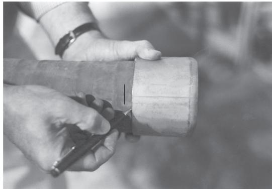
Hold the ferrule against the stem collar (sizes 1½" - 3" only). Using a small ruler or other measuring device, insert it between the stem and ferrule until it contacts the stem collar. Measure the depth at the end of the ferrule. Place a mark on the hose (the hose end to be assembled) that corresponds with this measurement.
