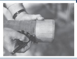
Slide the ferrule all the way onto the hose. Place a mark on the hose at the end of the ferrule. Move the ferrule 1/8" from the mark just made towards the end of the hose. Place a second mark on the hose at the end of the ferrule.
