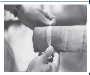
Accurately measure the hose O.D. with a diameter tape. Each end of the hose should be measured to guarantee the correct ferrule and die selection. Select the correct ferrule and die based upon the hose free O.D. just measured from the die chart. Make sure the hose end is cut square. If the hose is to be static grounded, follow hose manufacturers procedure for proper static grounding.
