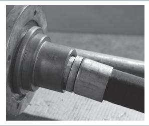
Insert the stem into the pusher so that the spacer ring just installed contacts the pusher.
