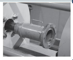
Install the 6" Main Pusher (**MPUSH600**) by sliding it onto the rod cam of the ram cylinder. Make sure that the pusher is all the way on the rod cap.
