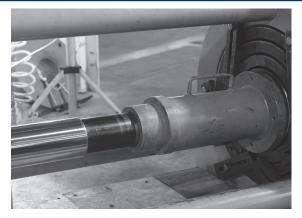
Depress and hold the button on the remote until the pusher meets the die face. When the extension contacts the die, release the button. Move the directional control lever to the "NEUTRAL" position. *Note:* The spacer ring will enter the die.
