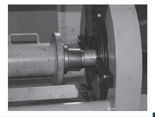
Put the directional control lever in the "FORWARD" position. Advance the cylinder forward until the end of the ferrule is near the die opening. Using a wooden board or metal pipe, lift the ferrule up. Jog the cylinder by depressing and releasing the button on the remote. This will allow the ferrule to enter the die slowly without contacting the die face.
