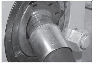
Install the required die holders ensuring that the seams between the die holder halves do not line up. The die holders are designed to fit one inside the other.
