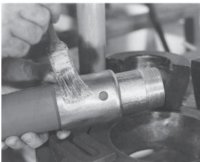
Lubricate the outside of the ferrule with Crisco® (recommended) or high viscosity oil or heavy duty grease.
