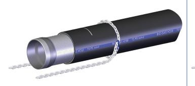
**5.** Place the cylinder end of the coupling inserter on the stud of the pusher plate as shown. Pull the chains through the holes in the coupling inserter as shown below. Be sure that the chains are pulled as tight as possible, and are locked into the narrow sides of the coupling inserter beam.
