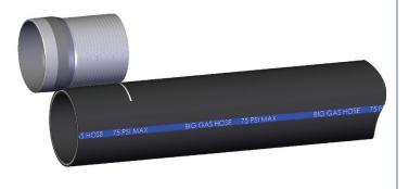
Lubricate the stem and ID of the hose with Dixon lube. Start the stem into the hose by hand so that the stem won't grab the end of the hose.
