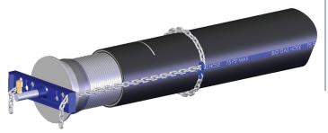
**6** Extend the cylinder to insert the fitting. If the coupling inserter begins to rock to one side, STOP extending the cylinder and reposition the chains as described in step 2.
