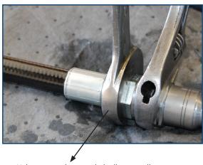
Using a wrench to crack the lines to relieve pressure
