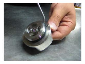
Change the O-ring (pos.14) on the threaded part to a new one. Use a greased O-ring.
