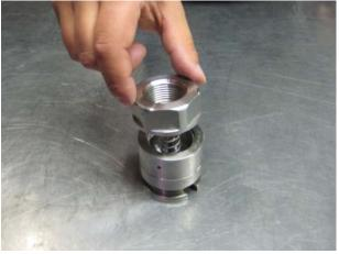
Remove the flat sealing. NPT-thread does not have a flat sealing.
