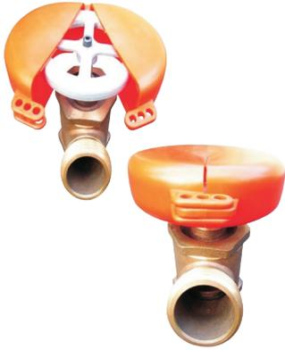
**Design:** Prevents unauthorised access to fire service and industrial valves. Device rotates freely around hand wheel to prevent valve wheel turning. UV resistant high grade PVC body is resistant to cracking, abrasion and extreme weather and temperature conditions. Has multiple padlock points.
