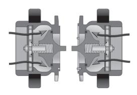
When the safety break-away couplings separate, it allows the poppets to close. The two poppets close rapidly, minimizing exposure to personnel and the environment.
